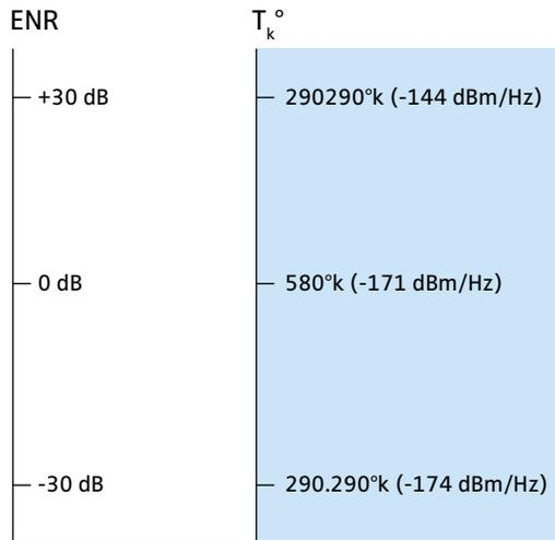
Calculating Noise Figure requires a knowledge of noise temperature, excess noise ratio (ENR) and noise power relative to 1 mW. The Noise Power Conversion Table is a graphic illustration of these relationships and is supported by mathematical definitions with example calculations.
